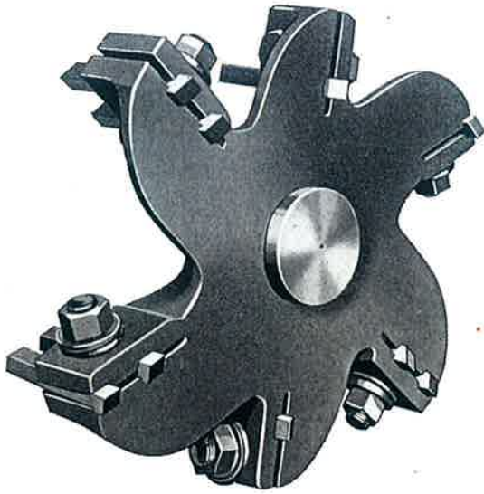
The improved type cutter head showing the bits, also the collar on the end of the shaft which serves as a gauge plate to regulate the depth of cut.
