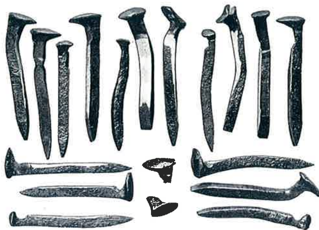
Examples of crooked and badly cut spikes pulled by the Spike Puller.
