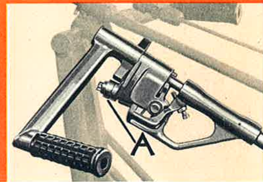
Here the overload release has functioned. The roller "A" has popped out from its notch in the operating lever and which no longer enables the operator to apply power to the sockets.
