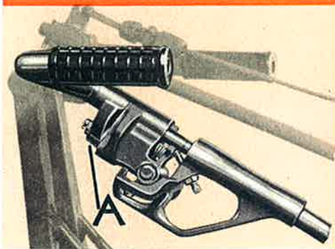
Here the connections to the operating lever are in normal position controlling the operation of the sockets. Note the position of the roller "A" in the notch in the operating lever.
