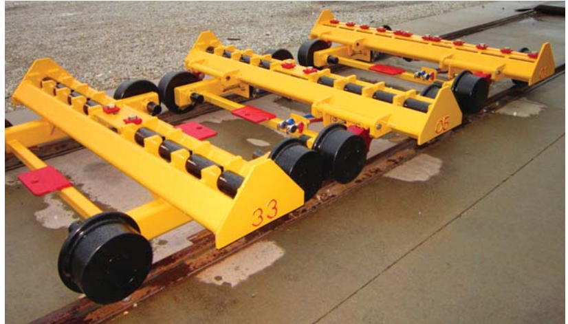
Mini Rail Train - cart without brakes, cart with brakes, and hold-down cart
