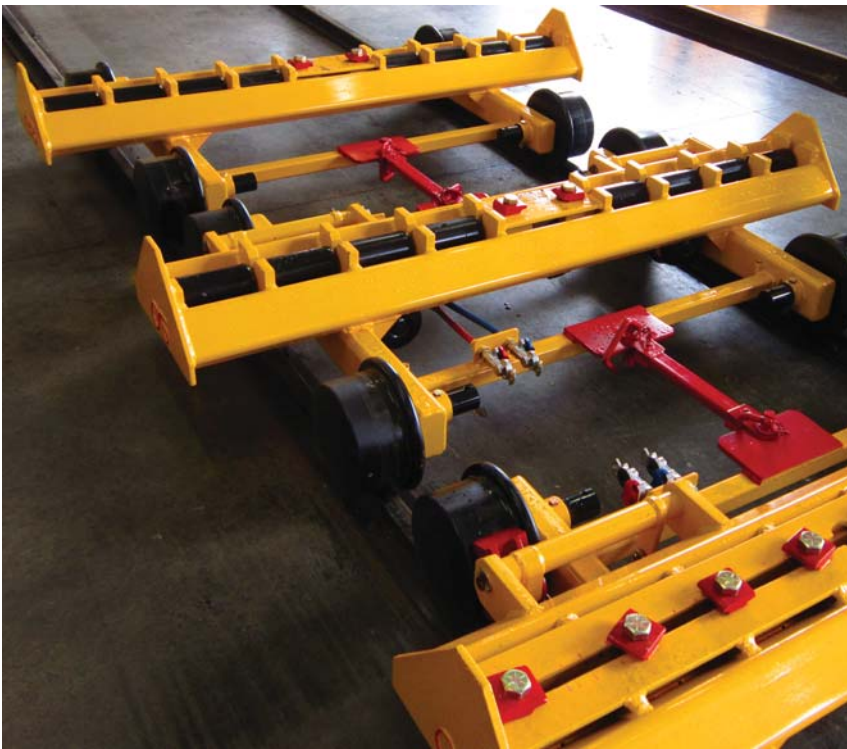
Tow bars connect the mini rail train during the transport to and from the work site.
