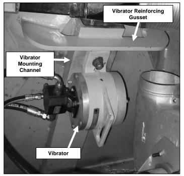
Figure 1 Vibrator Mounting Reinforcing Kit P/N 98410232
