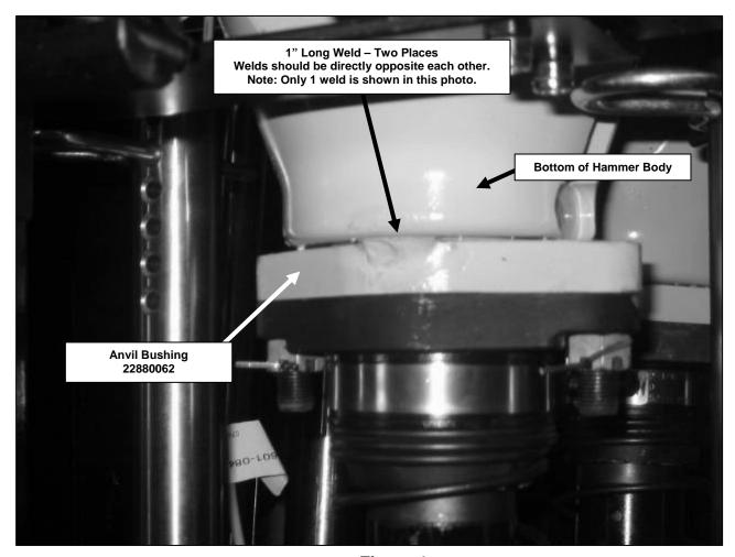
**Figure 1**Welding 22880062 Anvil Bushing to Hammer Body
