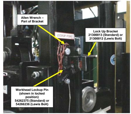
Figure 3 New Lockup Pin and Lock Pin Retainer installed on Roller Frame Kit 98350044 or 98350045
