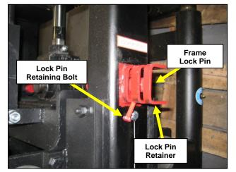
**Figure 1** Original Roller Frame Lock Pin P/N 54261101(Standard) or 54266240 (Lewis Bolt)
