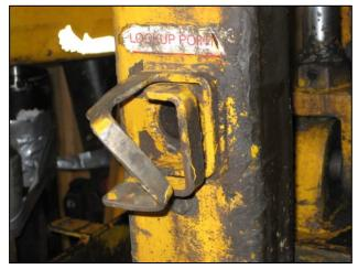
Figure 2 Damaged Lock Pin Retainer
