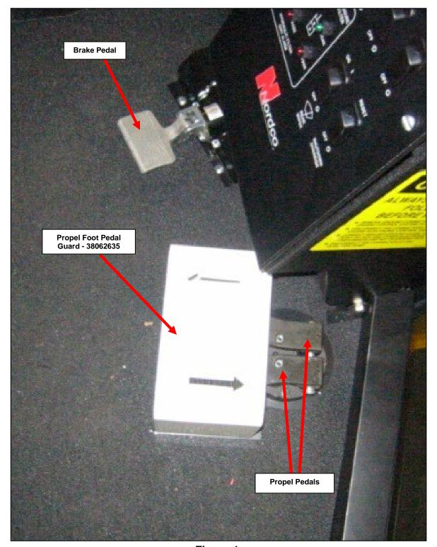
**Figure 1**98760061 Propel Foot Pedal Guard Kit installed in cab of TRIPP
