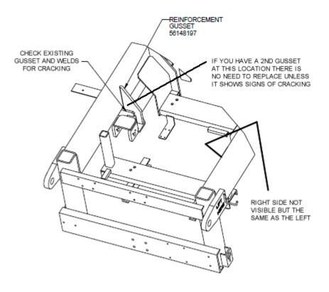
Figure 1. Rear Arm Inspection Area
