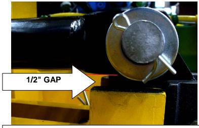
FIGURE 2. NEW STYLE LEVER 1/2" Gap between cylinder and frame weldment
