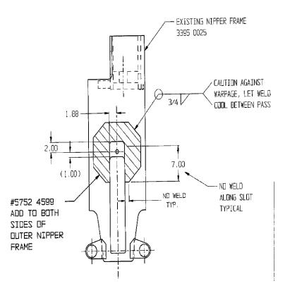
NOTE: The machine must be positioned over the tie before the nippers are lowered. If the machine is moving when the nippers are lowered the nipper frame can be shock loaded, which will result in failure of the nipper frame.
