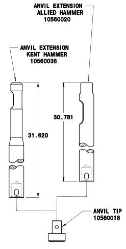
BOTH ANVILS USE A ROLL PIN, P/N 53643950 TO ATTACH THE TIP TO THE EXTENSION
