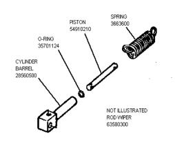
This cylinder is used on the spike driving gun assemblies of the listed spike drivers to feed spikes into the spike jaws. It is also used to operate the spike tray escapement cam on all spike drivers except the Model C. On the Anchor Applicator, it is used as the door open cylinder machines.
