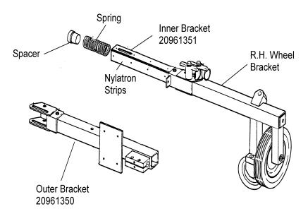
If the Nylatron strips require replacement, you do not need to return the entire Trak-Inspector. Only the inner bracket needs to be returned to NORDCO for repair.
