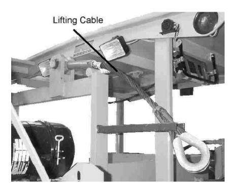
**Lifting Cable Installation**
