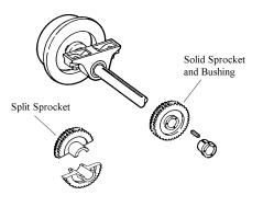
The following replacement axle assemblies have also been changed to incorporate the split sprocket:
