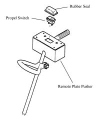
Second, the current switch is a "bezel mount" style switch. There have been some cases of the switch becoming twisted in the mounting hole and causing the switch to become jammed in the "ON" position.
