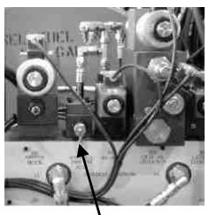
Joystick Pressure Reducing Valve on LH Manifold
