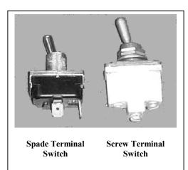
Anchor Applicators from s/n 680240 through 680250 used McGill screw terminal switches. These switches were found to be unreliable due to water being able to leak into the switch. These switches were replaced with Cutler-Hammer switches starting with machine s/n 680251. The Cutler-Hammer switches provide superior sealing against the weather. Any replacement switches ordered will be Cutler-Hammer switches.
