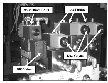
Figure 1 Typical D03 and D05 Valves
