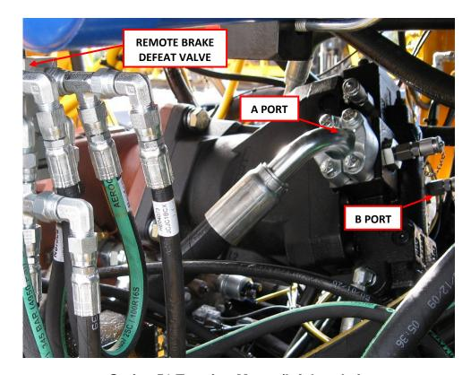
**Series 51 Traction Motor (left hand view)**
