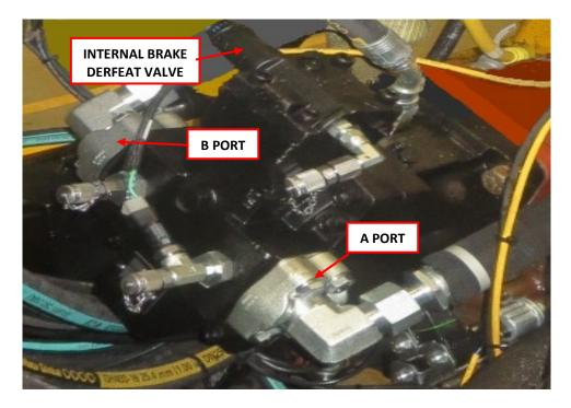
**Series H1 Traction Motor (right hand view)**
