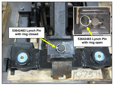
**Figure 2** Lynch Pin Claw Pin Retainer – p/n 53642483
