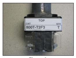
Figure 3 "Top" label faces front of cab
