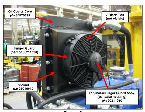
Figure 2 New Oil Cooler with Fan/Motor Assembly p/n 26740210 (24-volt)
