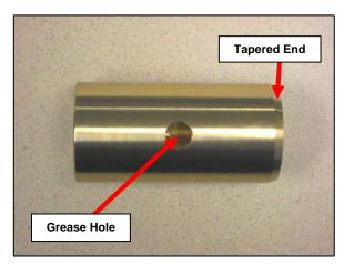
**Figure 1** 22034755 Guide Rod Bushing
