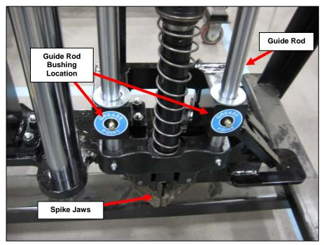
**Figure 3**Guide Rod Bushing Location
