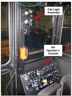
Figure 1 Cab Light Kit 98760056 installed in TRIPP cab
