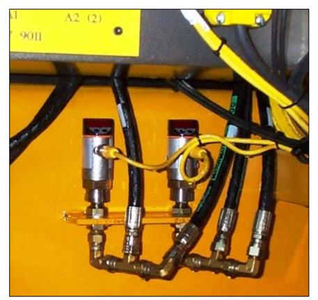
Figure2 Efector Propel Pressure Switches – 78893010 Included with Kit 98760062
