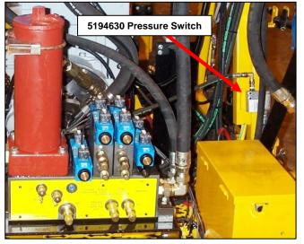
Figure 3 5194630 Barksdale Pressure Switch (used on machines s/n 791001-791006)
