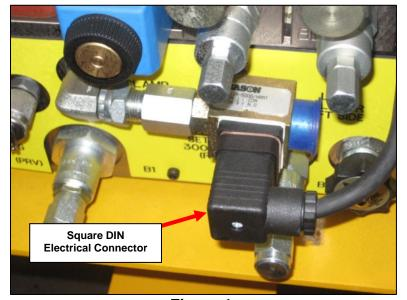
**Figure 1** 5194632 Nason Pressure Switch (used on machines s/n 791007-791062)
