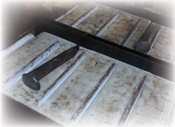
Four conveyor belts feed four spike trays, ensuring a steady flow of spikes to the driver guns.
