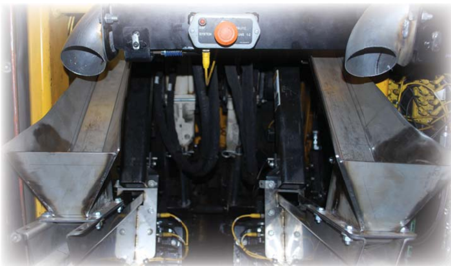
Four spike trays/baskets (two trays for each side) keep your spiking operations running smoothly.
