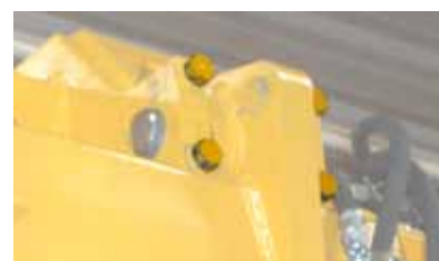
Easy-to-remove bolts mount the Workhead to the frame.
