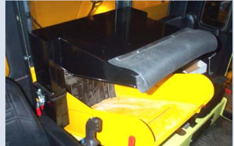
The Dust Hood Bumper Pad helps protect the machine operator.
