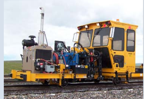
Kits are available for all major Nordco MOW machine types, including this Spring Clip Applicator.
