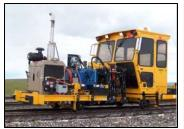
Spring Clip Applicator, one of several Nordco machines that can use the Foot Switch Mounting Bracket Kit.
