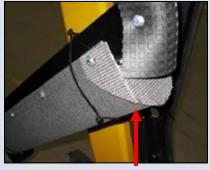
98410256 Spike Tray Dust End Cap attaches to the original Dust Chute. 98410257 is a complete Dust Chute & End Cap assembly.
